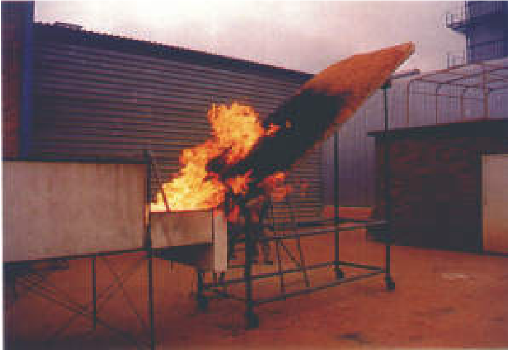
Figure 9: Spread of flame test Flames on thatch panel surface subsided
