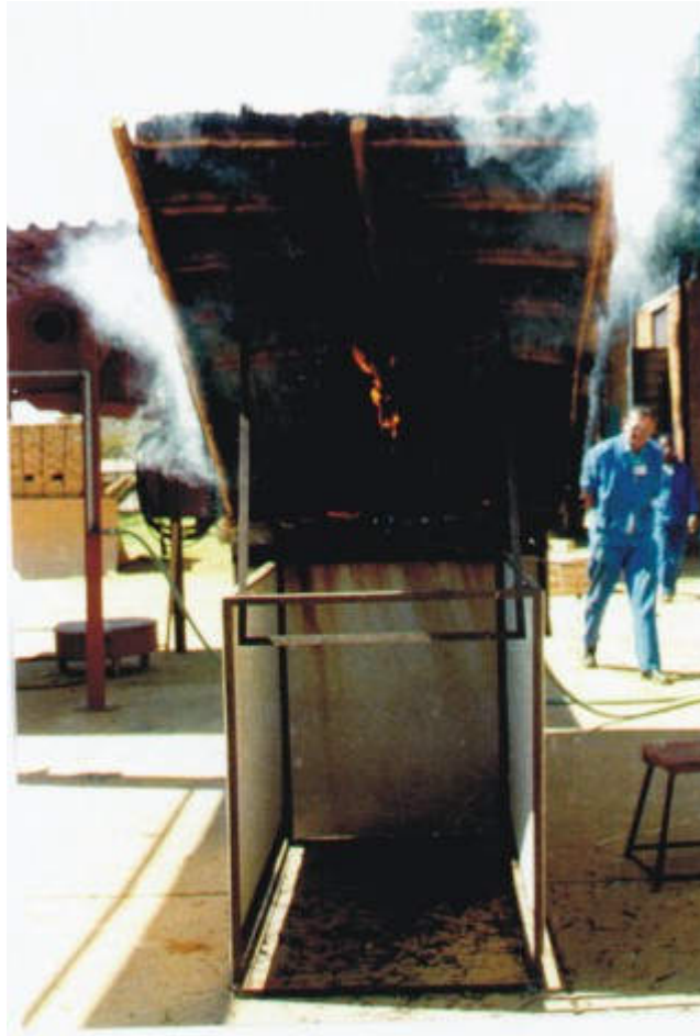
Figure 5: Intermittent flame test: Flaming on the underside of test roof during 8 th cycle
