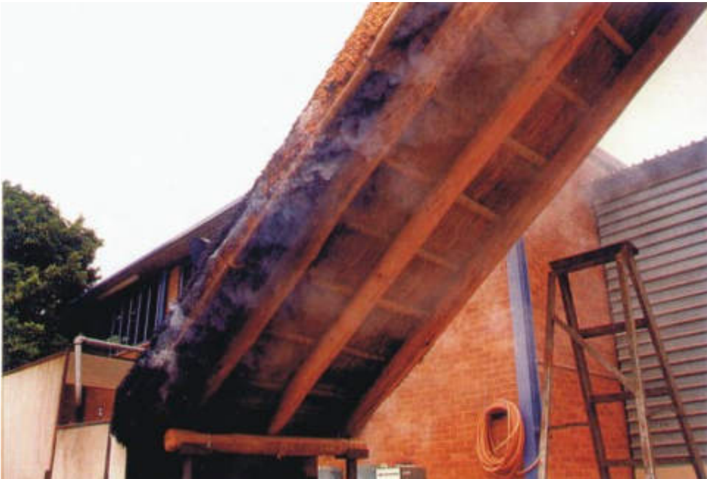
Figure 12: Spread of flame test Underside of roof immediately after burner extinguishment
