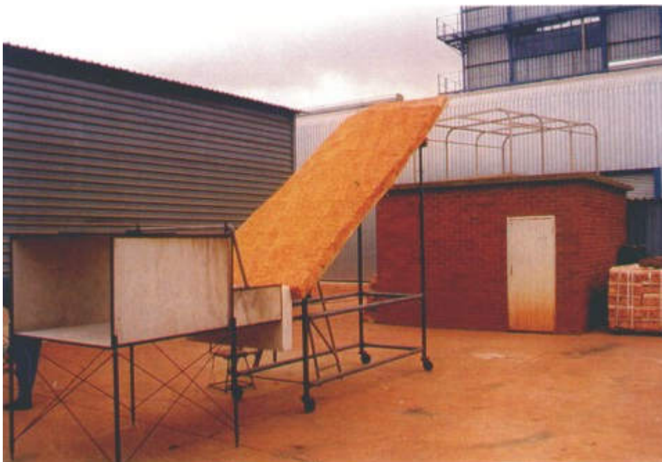
Figure 6: Spread of flame test: Test set up prior to ignition
