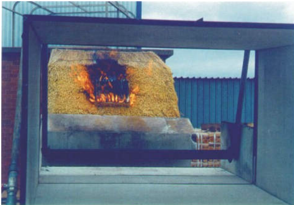
Figure 14: Burning brand test Placement of burning brand on thatch panel
