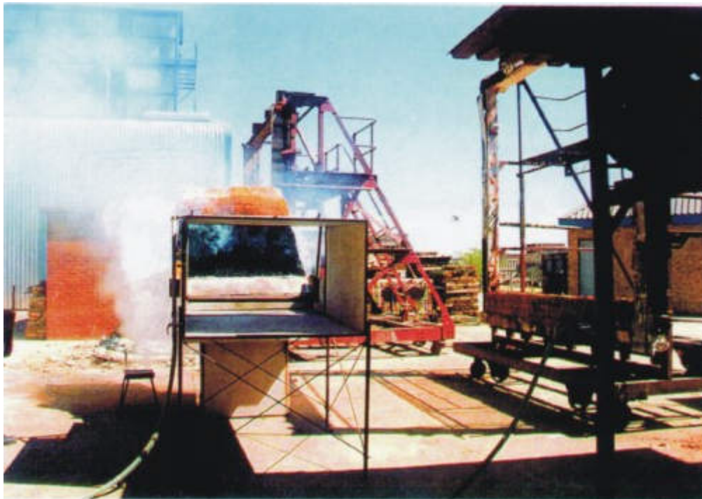
Figure 4: Intermittent flame test Thatch roof panel during a non flaming cycle
