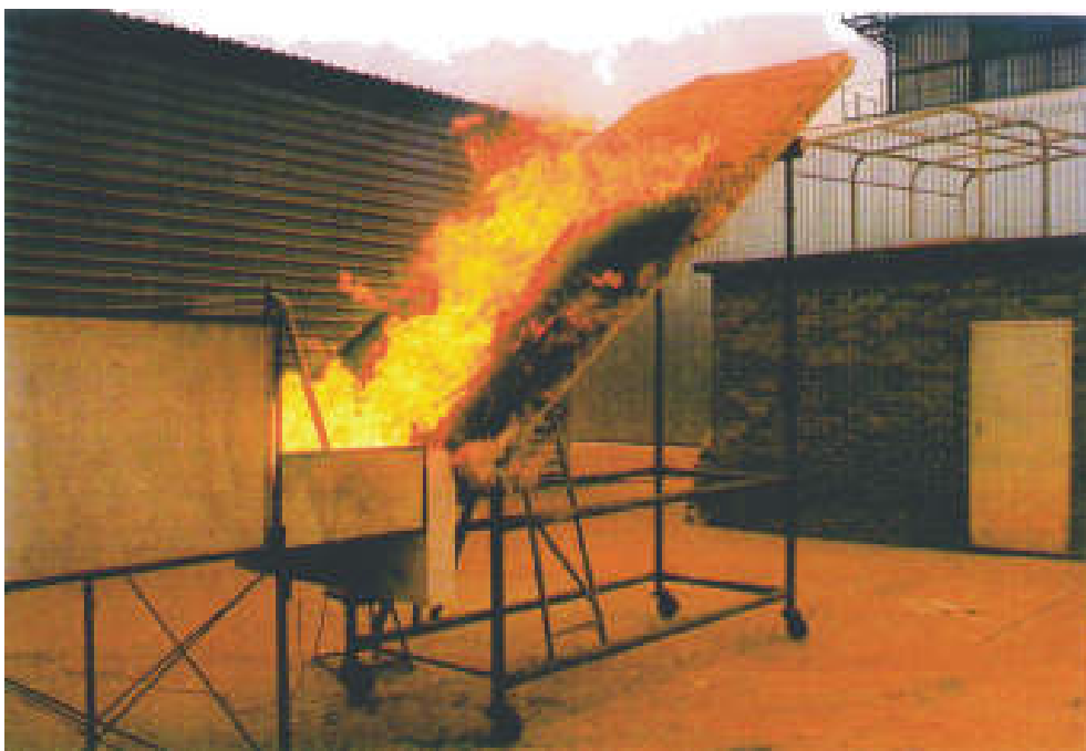
Figure 8: Spread of flame test Charring and small flames on surface
