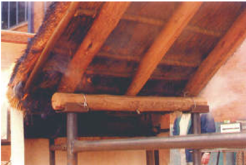
Figure 10: Spread of flame test Small flames on underside of panel
