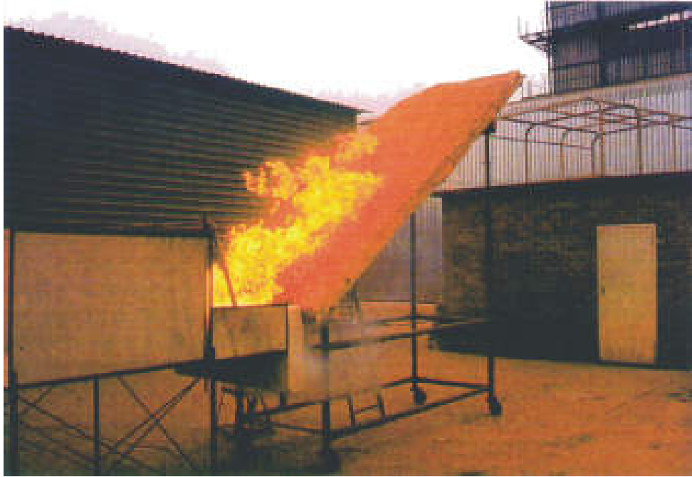
Figure 7: Spread of flame test Ignition of burner
