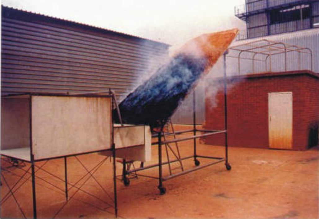
Figure 11: Spread of flame test Burner extinguished
