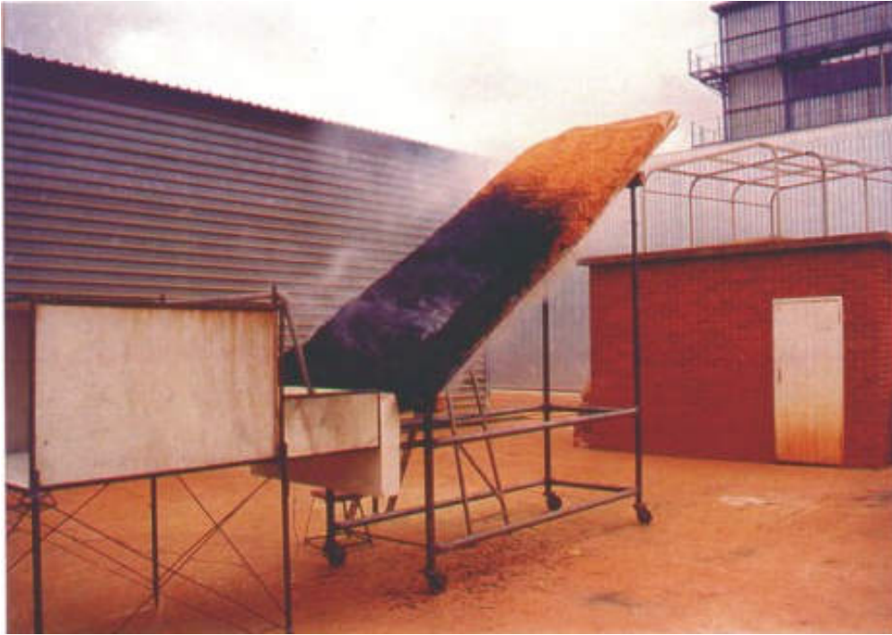
Figure 13: Spread of flame test Glowing on bottom edge disappeared
