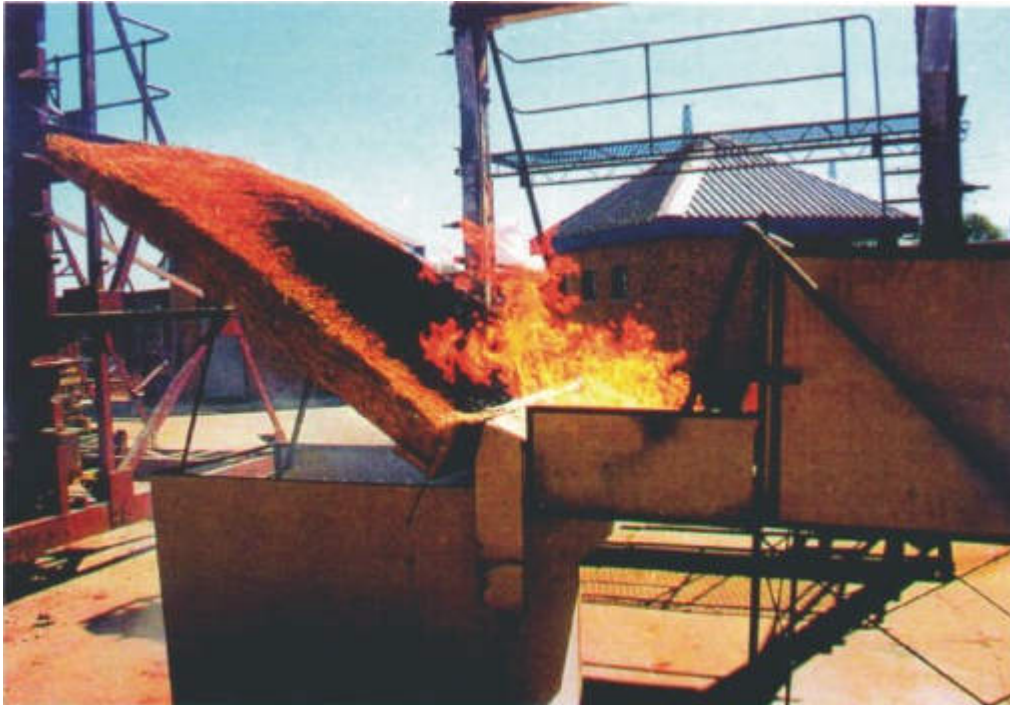
Figure 3: Intermittent flame test Test set up during a flaming cycle
