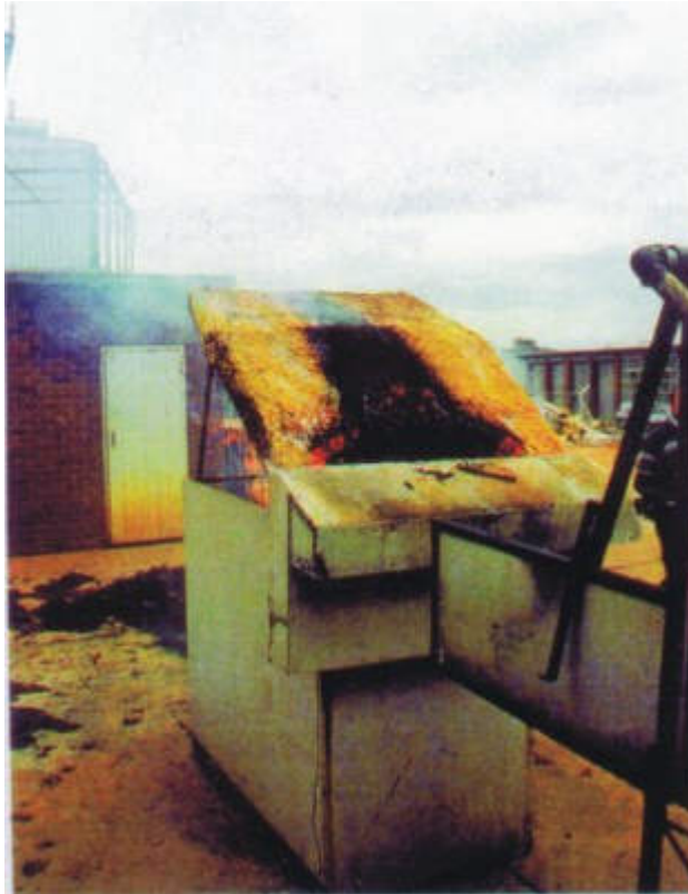
Figure 15: Burning brand test Glowing and small flames in lower region of panel
