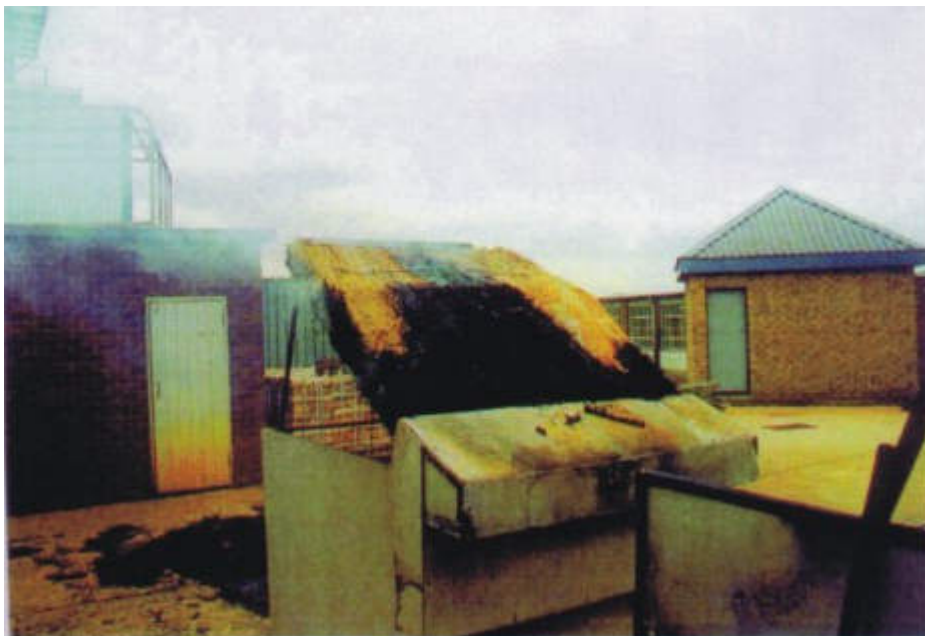
Figure 16: Burning brand test Effect on brand deceased, visible glowing disappeared
