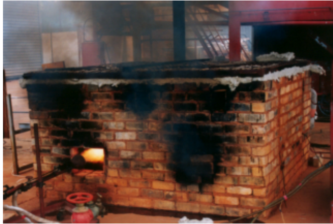
Figure 6: Diesel burner on righthand side in operation
