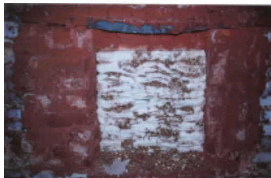
Figure 6 : Photograph of the interior of the DJ Fire Pillow Fire Stop System showing the effects of two hours exposure at 1150 degrees celcius
