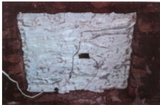
Figure 5 : Photograph of the DJ Fire Pillow System at end of test
